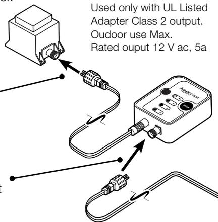
This timer features easy, single-button programming, durable weatherproof construction, and quick-connect weatherproof connections.
