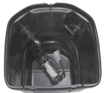
Ex. 15 One adaptor threads directly into the pump, the other threads directly into the bulkhead on the back of the skimmer. Apply silicone or Teflon tape (not included) to the threads of the fitting. NOTE: One pump shown. Your installation may have two pumps.
