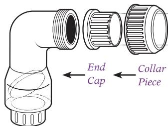
*Slide collar piece over PVC, then glue pipe end cap to PVC tubing. Slide collar up to check valve and hand tighten. It's as simple as that!*
